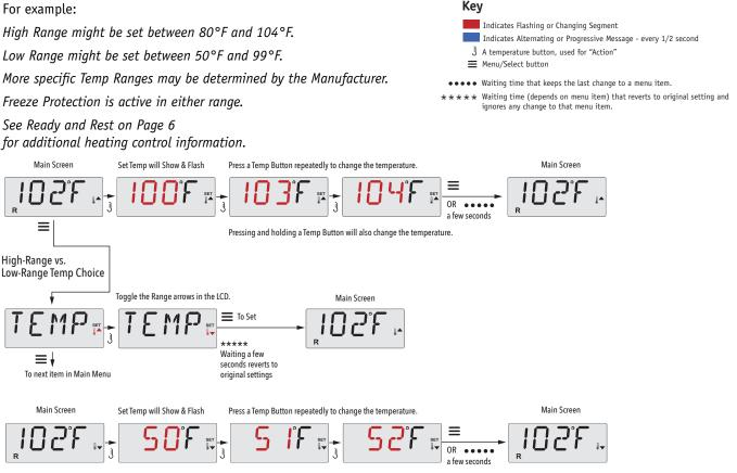
Pressing and holding a Temp Button will also change the temperature.
