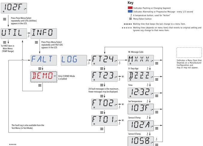
Waiting a few seconds inside the Fault Log Menu will allow the screen to return to normal operation.
