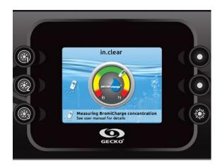
When BromiCharge is added the indicator will move slowly to the right. When water is added to the spa the indicator will move to the left. To obtain a good level of BromiCharge, start the pumps and add the specified amount of BromiCharge\*\* and allow 5 minutes for the indicator to adjust before adding more.
